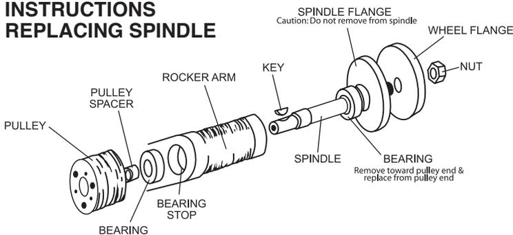
5. Place a pipe slightly larger than the arbor shaft, over the pulley end of the shaft and against the **inner race** of the bearing.
