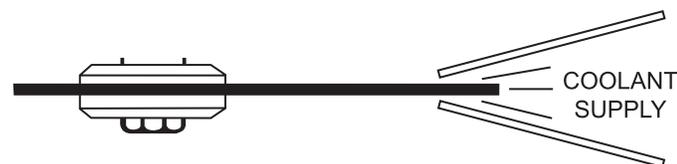
When coolant is directed evenly on both sides of the wheel, edge remains square and makes square cuts.
