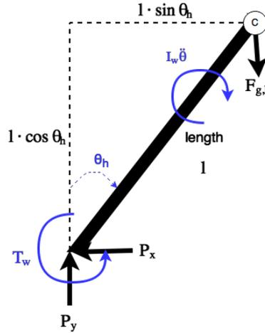
Figure 2: Free body diagram of human
