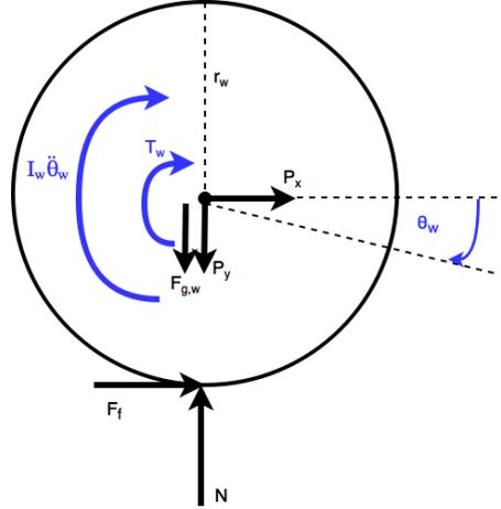
Figure 1: Free body diagram of Segway wheel
