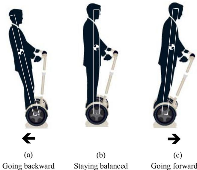
Fig. 1: The balancing ability of a Segway
