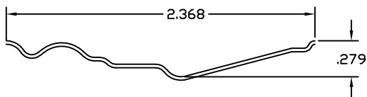
EMBOSMENT PROFILE SECTION A-A SCALE 16X
