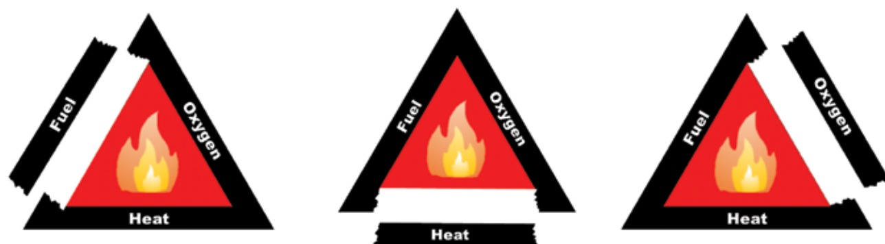
Figure 3.4. Removing any element in the fire triangle will stop the combustion process (Wildfire Planning International and Wildland Professional Solutions)
