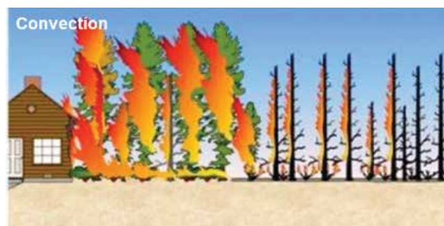
Figure 3.6. The convection heat transfer process from vegetation to a structure during a WUI fire (Partners in Protection Association)
