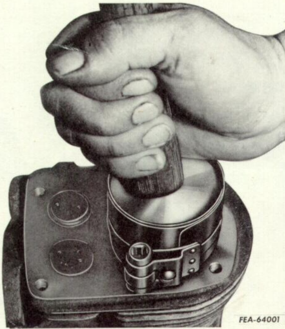
Illust. 1-20. Installing piston assembly.
