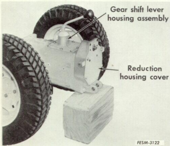
Illust. 2-24. Power train supported for disassembly.
