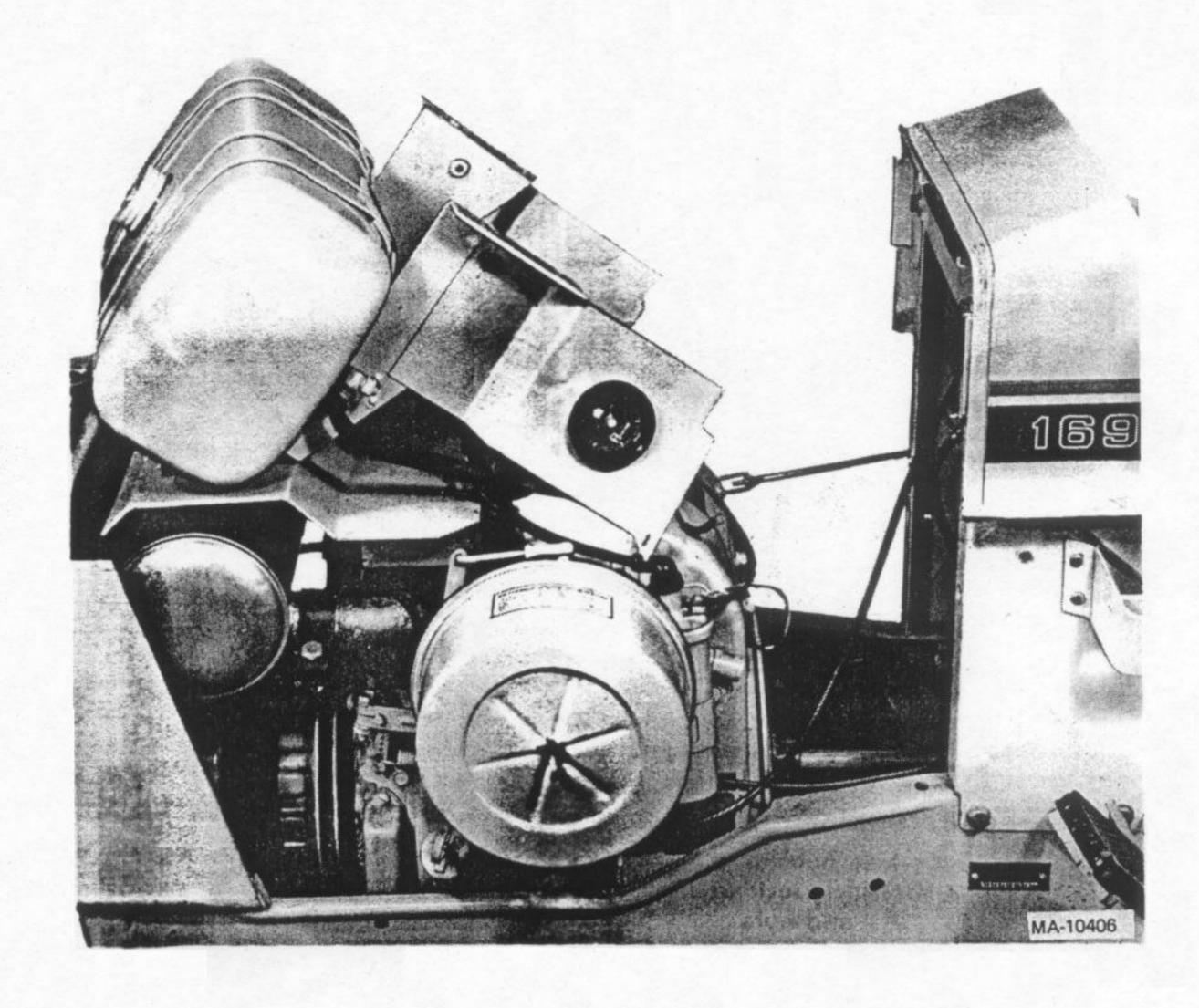
NOTE: Remove the fuel tank and extension panels as an assembly.
