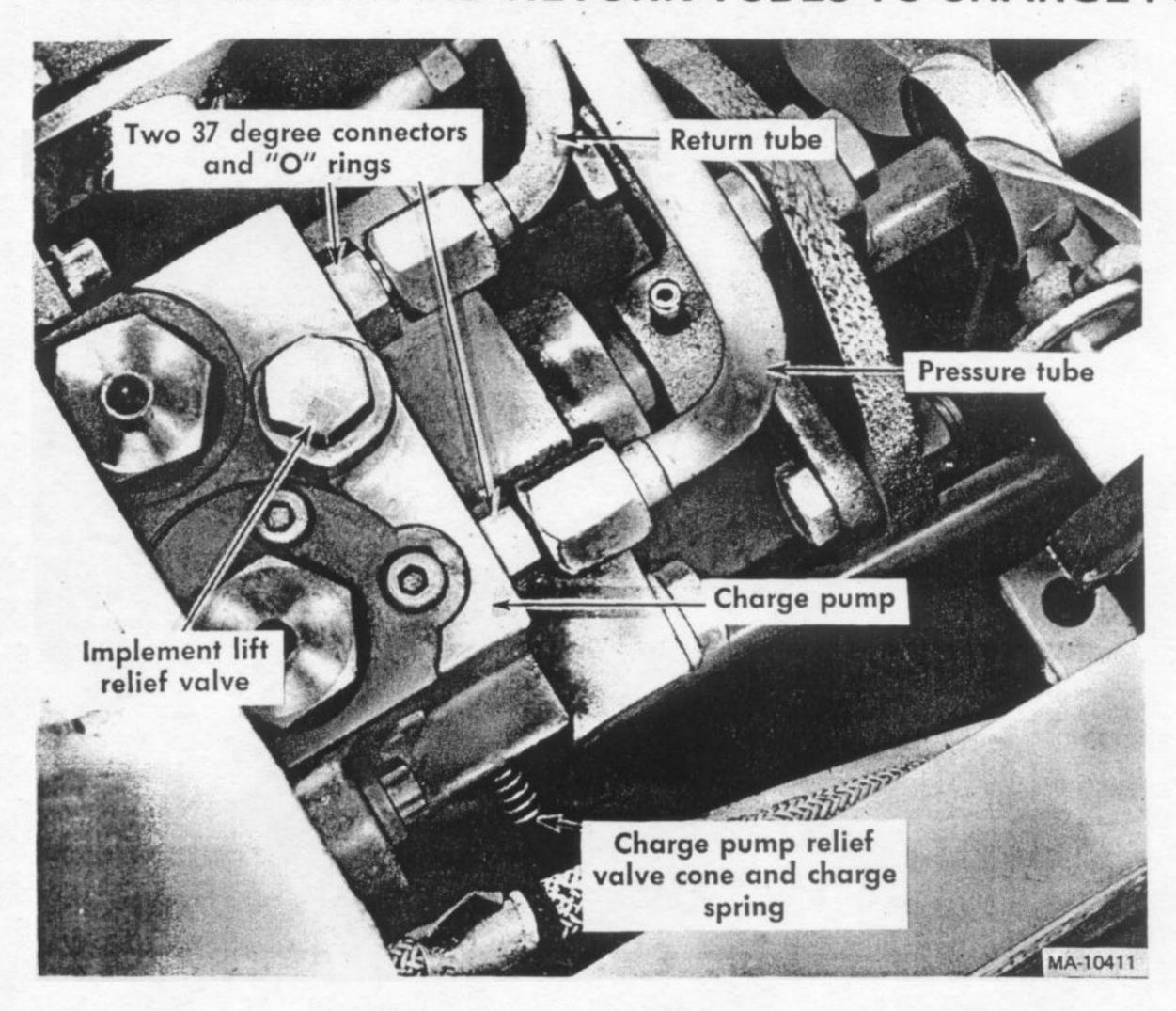
Remove the plug from the implement lift relief valve and remove the charge spring from the valve. (DO NOT DISCARD THIS SPRING.) Install new spring provided in the package. Spring wire is 1/16-inch diameter. Replace the plug.
