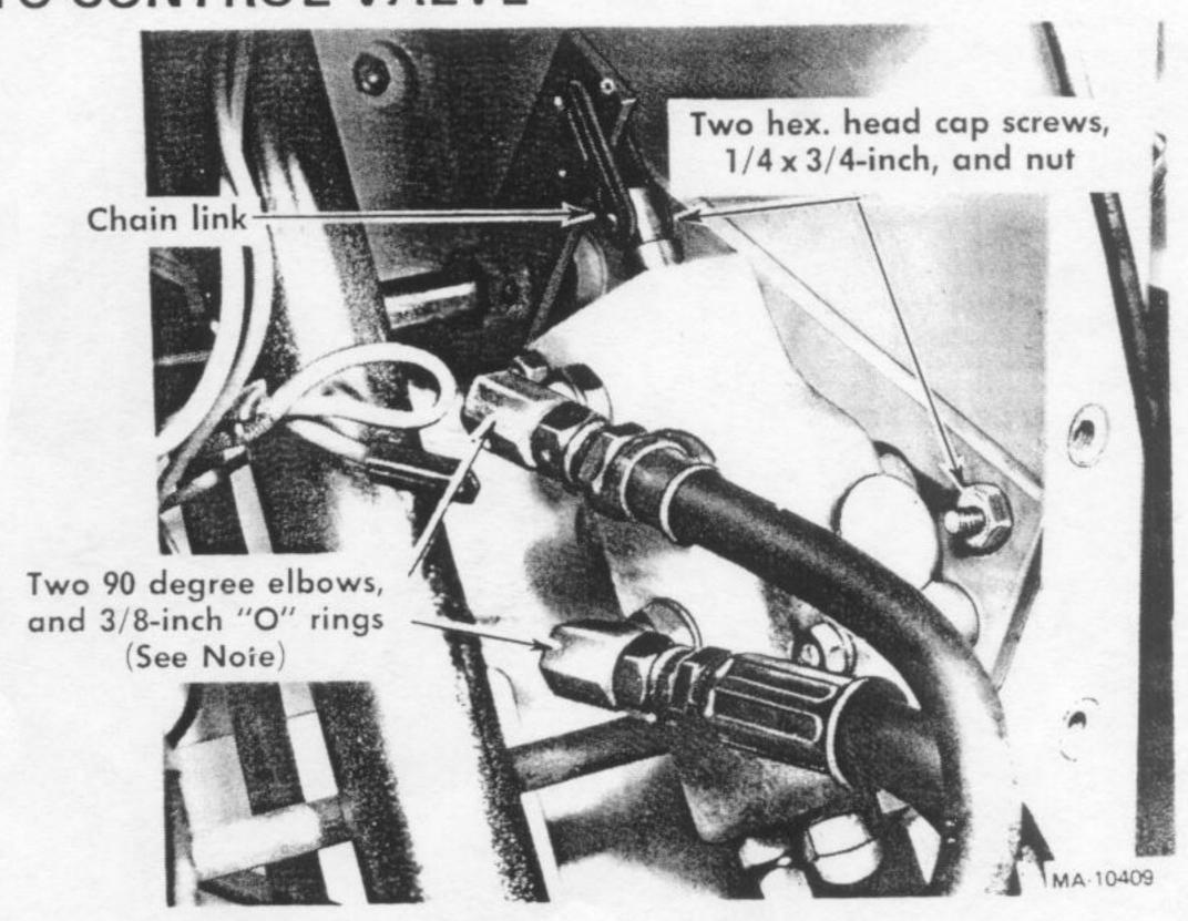
NOTE: Longer hose fits into the upper fitting on the control valve.
