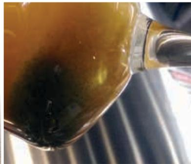
Hop particles after settling
