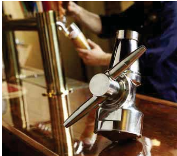
Alfa Laval Rotary Jet Mixer blends in the natural flavours and mixes CO 2 and water into the beer.
