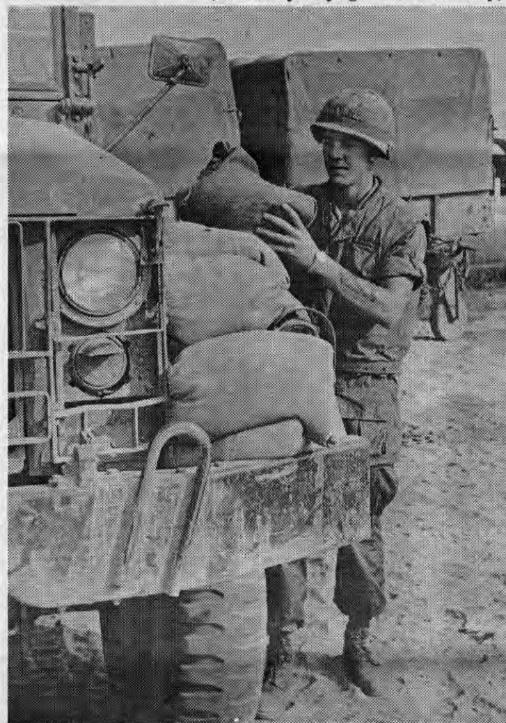
SANDBAGGER—Marine Pfc Robert L. Franklin, (Woodbury, N.J.), stacks sandbags on the lead truck before starting on a Marine convoy. Franklin is a volunteer mine truck driver with Marine 3rd Motor Transport Bn. The mine truck is sandbagged heavily to ward off injuries in the event a mine is detonated on the convoy route.
