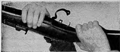
32.3(1) Swing trigger guard away from trigger housing.
