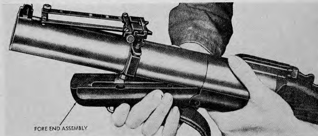
37.6 Removing or installing the fore end assembly.
