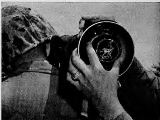
26.5(5) Gives rocket slight rotary twist to insure effective electrical contact.
