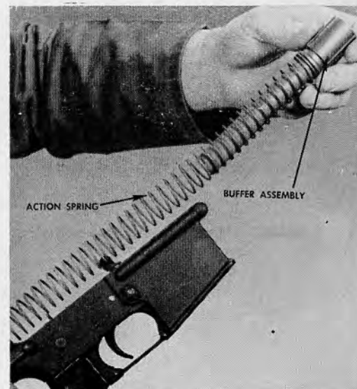
34.18 Removing the action spring guide assembly and action spring.
