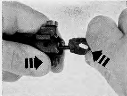
35.19 Replacing extractor and ejector.
