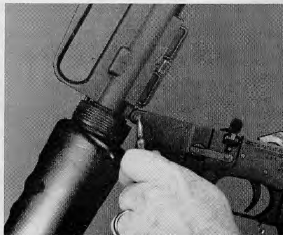
34.4 Pressing the receiver pivot pin to the right.
