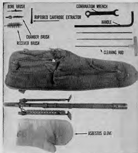
36.33 Cleaning equipment, spare barrel, and spare barrel case.
