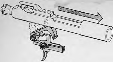
34.31 Cocking (showing action of the disconnect).
