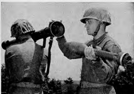
26.5(2) Loader presses down on contactor latch to clear the way for rocket.
