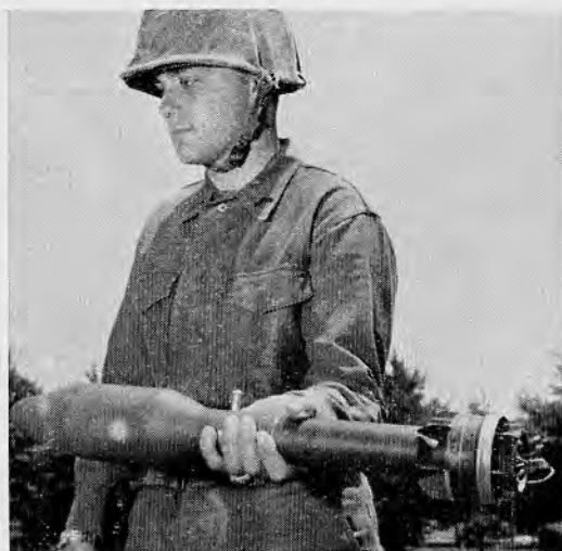
26.5(1) The loader grasps the rocket in his left hand and removes shorting clip from contact ring assembly.
