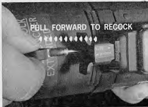
33.11 Recocking during immediate action.
