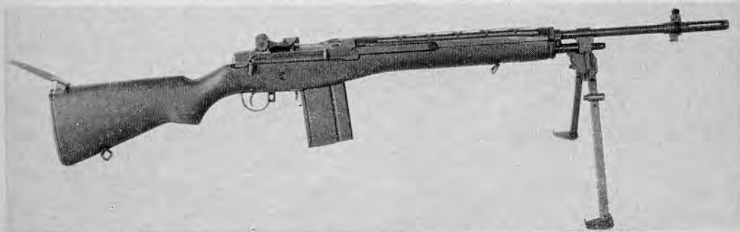
35.40 The M14 Rifle, showing Rifle Bipod M2, mounted in firing position.
