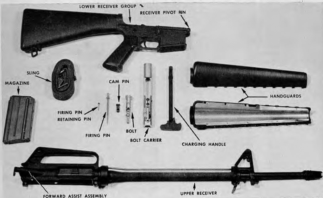
34.14 Field stripping completed.
