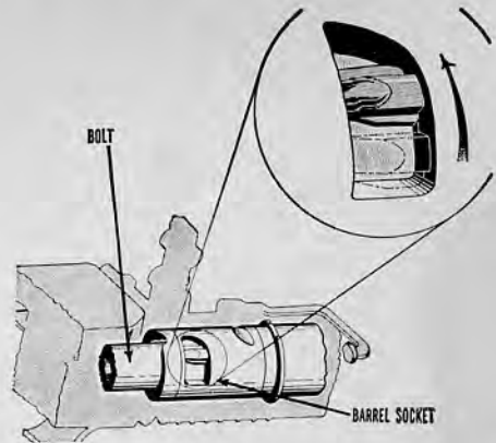
36.30(b) Unlocking (upper bolt locking lug rotating counterclockwise in bolt locking cams in the barrel socket).
