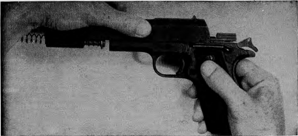
24.5 Field Stripping (Removal of Slide Group).
