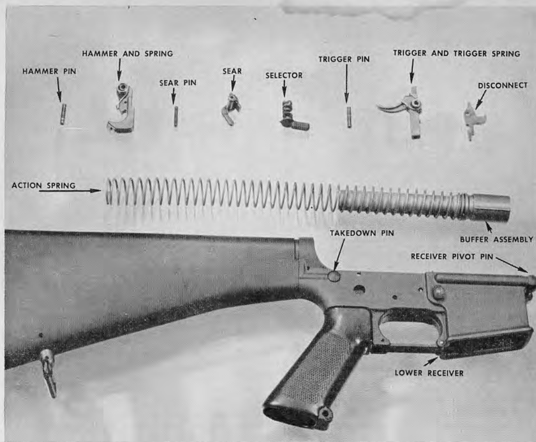
34.23 The lower receiver group disassembled in detail.
