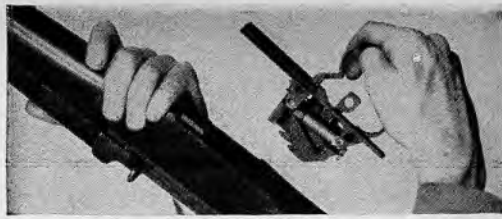
32.3(2) Pull out the trigger housing group.
