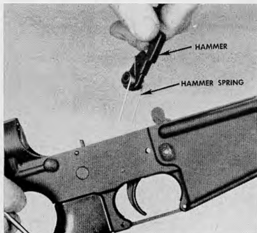
34.17 Removing the hammer and spring.
