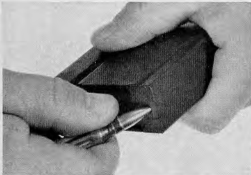
35.15 Removing the base of the magazine.
