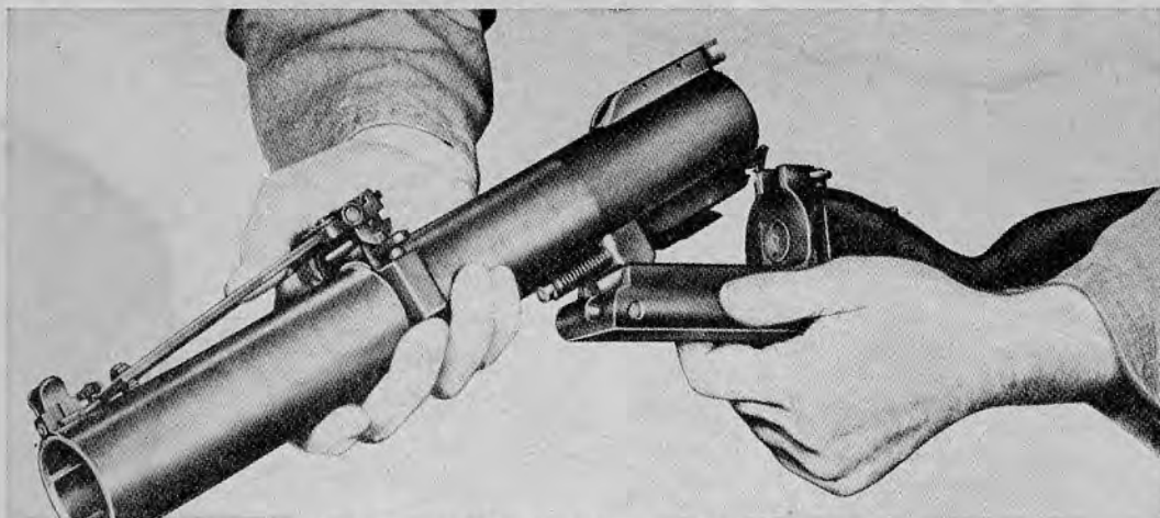
37.7 Removing or installing the barrel group.
