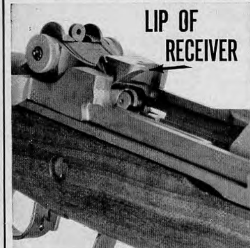
35.36 Points to apply lubriplate.
