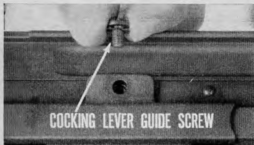
36.20(a) Unscrew and remove the cocking lever guide screw.
