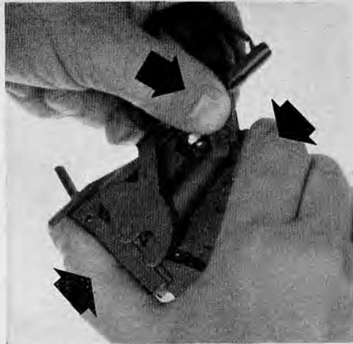
35.22 Seating the trigger pin.
