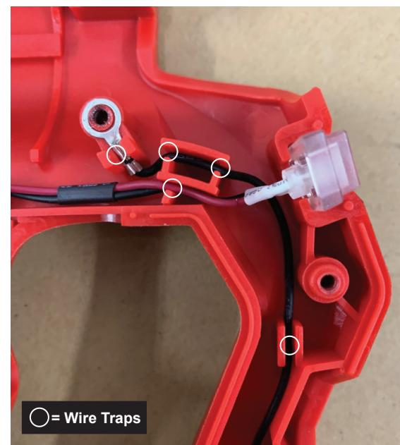
As an aid to reassembly, take notice of wire routings and position in wire guides and traps while dismantling tool.
