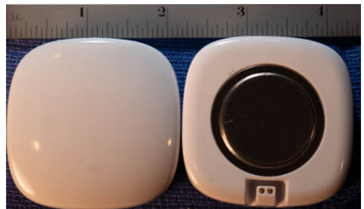
Figure 1: Image of heating units used in the study. The left image shows the side of unit that faces away from the skin. The right image shows the metal heating plate that is one inch in diameter. The heating plate rests on the skin over the area of pain.
