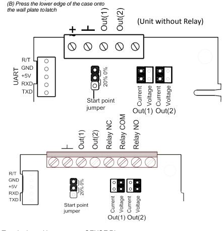
Terminals and jumpers on aSENSE RL. The darker positions are default settings. Terminals and jumpers are located under the toppart.
