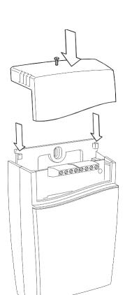
The top part is pushed under the locking hooks of the wall plate and is secured with a screw
