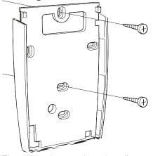
The wall plate is screwed onto the wall The screw head diameter should be **max 7,5 mm** The screw head height should be **max 2,5 mm**
