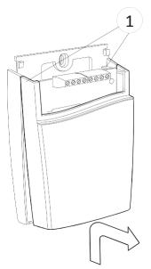
Fold the front part with the lid forwards and loose it from the hooks (#1)
