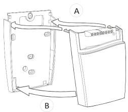
(A) Put the top tabs of the front part into the top holes of the wall plate.
