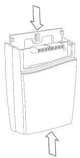
Push the front part with the lid upwards while keeping the wall plate steady
