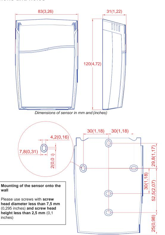
Dimensions of mounting plate in mm and (inches)
