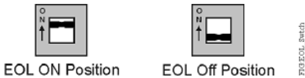
Figure 14: End-of-Line switch positions
