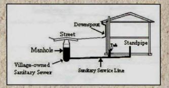
Precautions: If the elevation of the back-up is high enough, the back-up will be seen in the next higher opening (basement toilet or tub) and structural damage to the home may occur.
