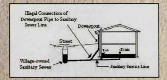
Blockages from grease or debris can cause partial or complete blockage of the sanitary sewer service.
