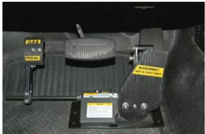
The above images are two examples of adaptive equipment; hand controls with a steering wheel and left foot accelerator.
