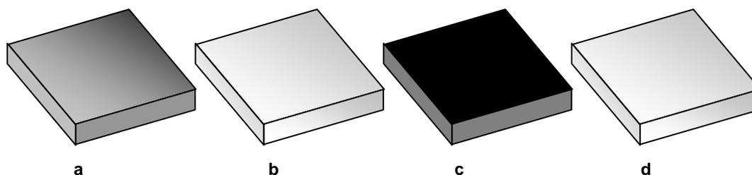
**Figure 1.** **a.** defrosting tray, **b.** defrosting tray covered in aluminum foil, **c.** white Styrofoam plate, **d.** blackened Styrofoam plate
