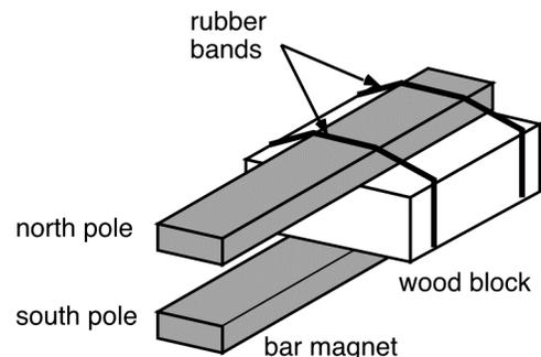
**MAGNET:** Sandwich a small wood block between two bar magnets. Secure the arrangement with rubber bands as shown. Note that the magnets are antiparallel: opposite poles face each other.
