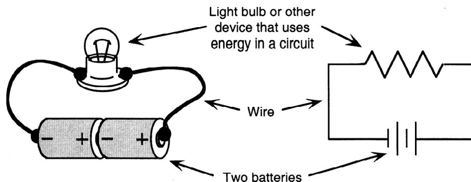
Using a bare bulb (out of its socket), one battery, and **two** wires, try lighting the bulb in as many ways as you can. On a separate sheet, sketch at least two *different* arrangements that work. Also sketch at least two arrangements that don't work. Be sure to label them as "works" or "doesn't work."
