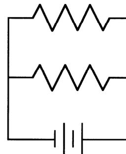
**Figure C.** Parallel circuit
