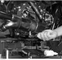
The AC header pipe is loosely secured to the transmission mounting bracket using the stock hardware, some blue Permatex threadlock, and a 9/16" socket.
