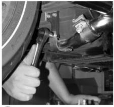
The stock crossover pipe (with clamp) is then loosely resecured to the stock mounting bracket using the stock hardware, some blue Permatex threadlock, and a 1/2" short socket.
