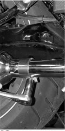
Now that the entire system is installed on the bike, tighten all the hardware, starting at the heads, and working your way back. Use a 9/16" socket on the muffler exhaust clamps.
