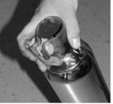
The stock muffler exhaust clamps slip onto the American Custom mufflers. Be sure they are positioned so their bolt is facing in and the nut is facing down.
