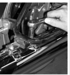
Slide the AC mufflers onto the AC header pipe and lightly attach them to the stock rear mounting brackets using the stock hardware, some blue Permatex, and a 1/2" socket.
