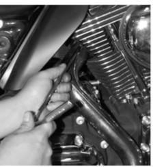
Using the stock exhaust flange nuts, John loosely attaches the AC header pipes to the engine using a 1/2" socket. He does this by tightening both nuts down evenly, front to back.
