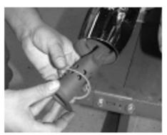
These mufflers can be used with or without baffles. To install them, slip the provided gasket over the baffle, then slide the baffle into the open end of the muffler.
