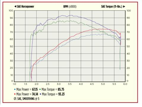
increased quite a bit and so did the power output. We got 74.14 hp and 93.23 ft-lbs. of torque, for a gain of 7 hp and almost 8 ft-lbs. of torque over the stock pipes. And we didn't touch the EFI fuel or ignition settings. This is the run you see on the accompanying dyno chart.
