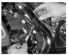
The stock rear header pipe heat shield is lightly attached next using a flat-bladed screwdriver and the stock clamps.
