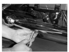
Once the stock crossover heat shield is installed, correctly position all the shields and secure them to their respective pipes using a flat-bladed screwdriver on the stock clamps.
