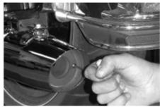
To secure the baffles to the mufflers, tighten the AC-supplied bolts and lock washers to the interior of the muffler using the optional AC 1/8" T-handle Allen.
