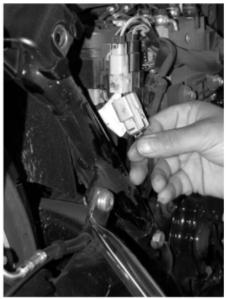
With the header pipes in place, the O<sub>2</sub> sensors can be reattached to their stock connecters, behind the ABS module, under the right-side cover. Their wires are then wire-tied to the frame.
