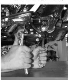
The stock right floorboard is reinstalled using the stock mounting bolts and some blue Permatex. Use a 5/16" Allen and 9/16" wrench to torque the hardware to spec.
