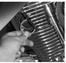
After removing the stock exhaust gaskets from both exhaust ports, John installs new ones (not included) into both heads.
