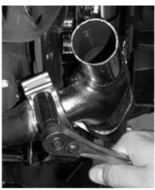
The stock crossover exhaust clamp can now be correctly positioned on the pipe and loosely secured using a 5/8" deep socket.
