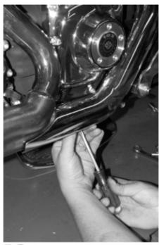
After wiping down the whole exhaust system with glass cleaner, the stock heat shield for the front header pipe is loosely installed using a flat-bladed screwdriver and the stock clamps.
