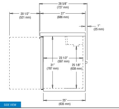
**IMPORTANT NOTE**: Models are completely front breathing and take in and exhaust air through the front grill. A clearance of 1" on the back and 3" on the sides is recommended.
